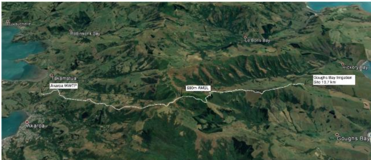
Figure 6-4 Pipeline Route to Goughs Bay Irrigation Site (image courtesy of Google Earth)
