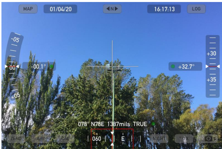
Figure 1 – Typical digital inclinometer reading of a 12m pole on sports field number one.
