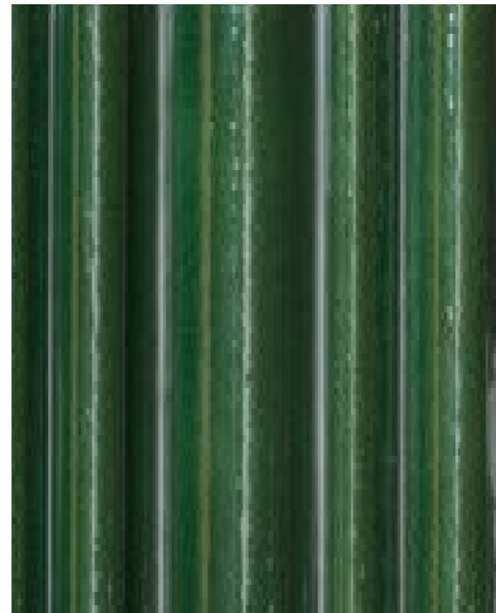
Sinusoidal ceramic profile roughly 2-3 times the scale of corrugated iron
