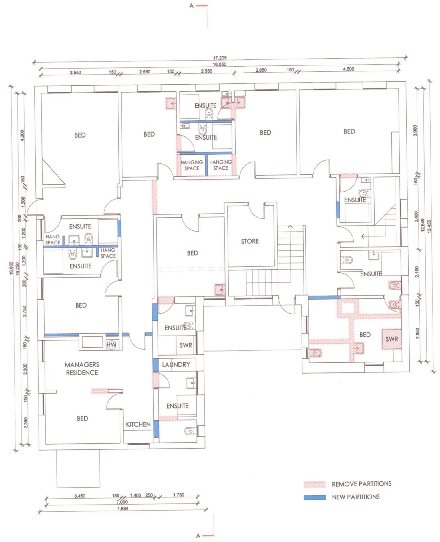
FIRST FLOOR DEMOLITION PLAN
