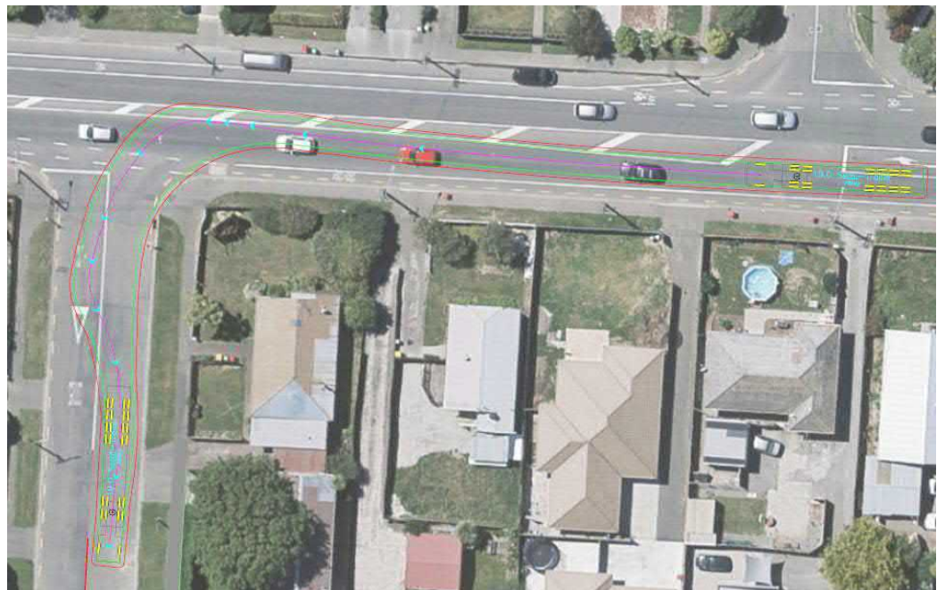
Figure 6 Tracked path of semi-trailer accessing Lydia Street
