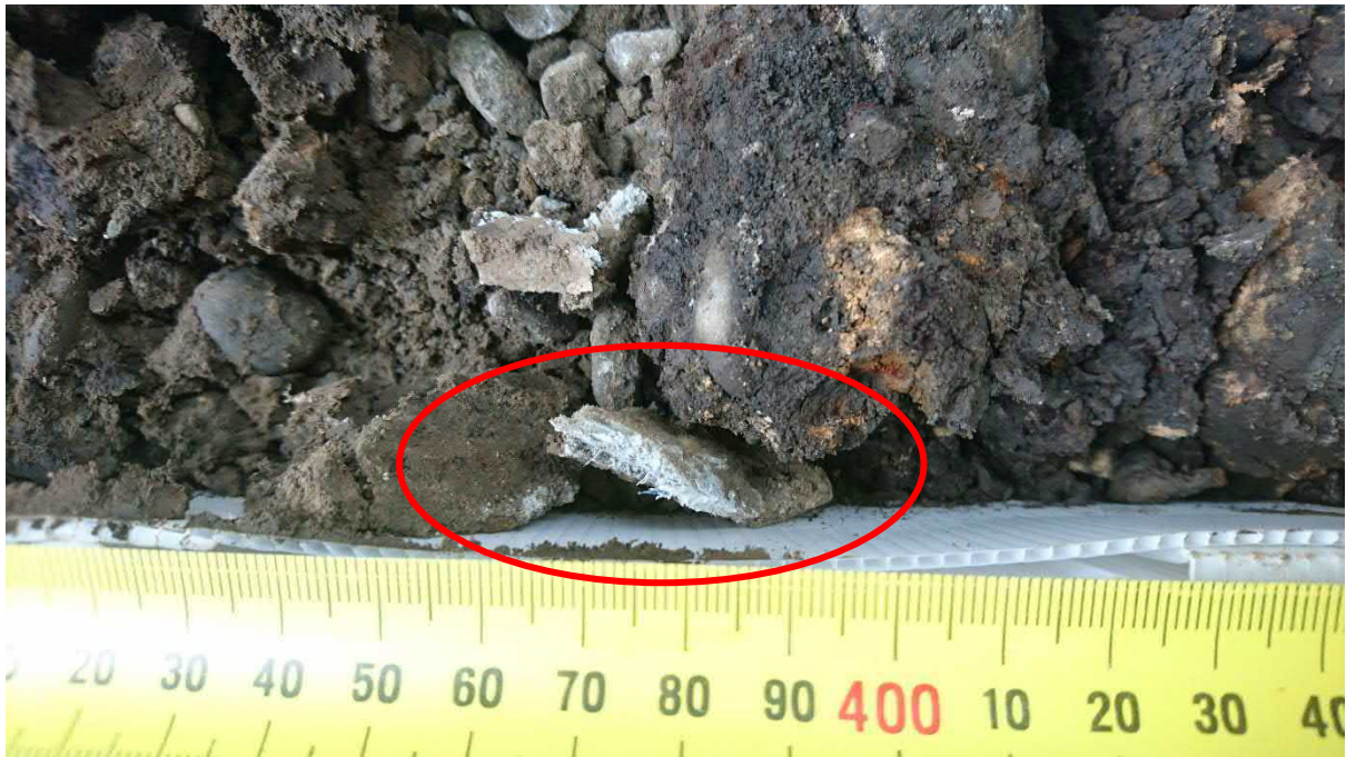
Photograph 5 – example of asbestos containing material (cement board materials) (Borehole 111 at 0.7 m bgl).
