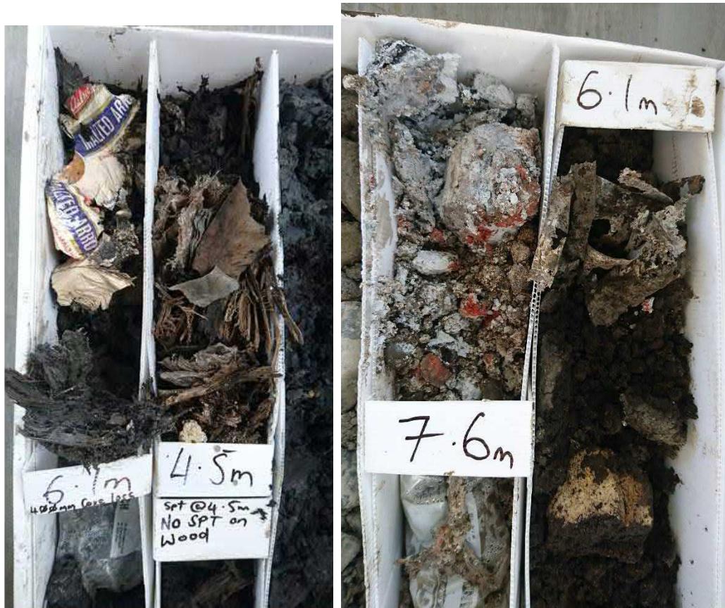
Photograph 4 – examples of landfill materials.
