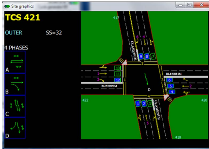
Figure 2: Blenheim Road / Clarence Street Signal Phasing
