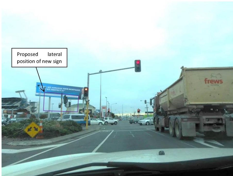
Photograph 11: Driver's View from Ferry Road - At Maximum Deceleration Rate Distance
