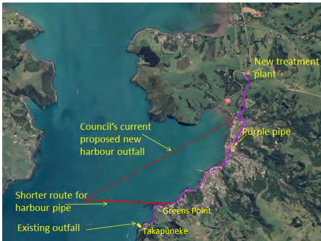
Figure 1 Cost-effective harbour outfall options
