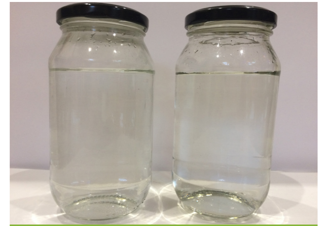
Figure 4 - Tap water (left) and reclaimed water from the Turangi wastewater treatment plant (which uses membrane filtration as proposed for Akaroa).
