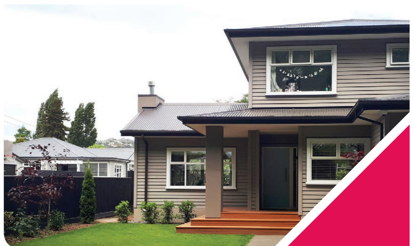
Contemporary house using character details such as weatherboard cladding, corrugated iron roof, clear front entry with a modern porch and large windows facing the street
