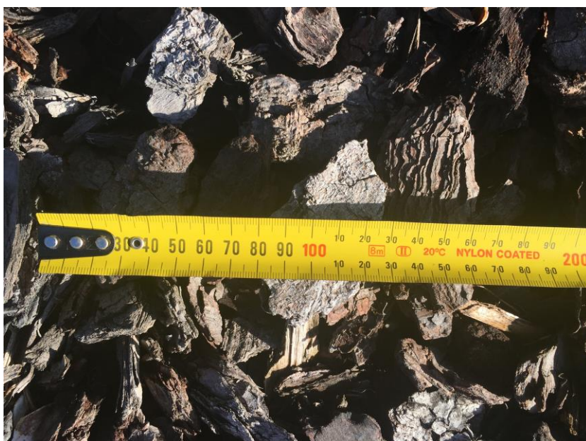
Photo: Premium bark nuggets, homogeneous and well graded, with a particle size between 32 and 55 mm
