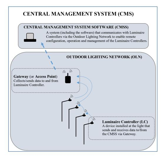
The Outdoor Lighting Network is an Itron Network Solutions mesh network.
